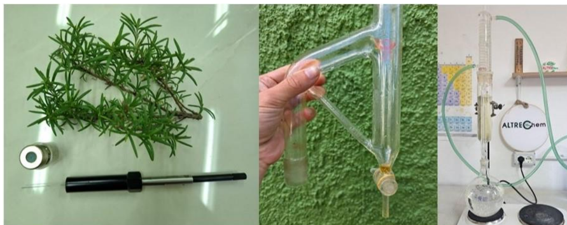
Figure 1. Extraction of rosemary by using HS-SPME, HD and SE techniques.
